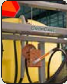
Standard boom height controlled by winch or optional hydraulic cylinder
