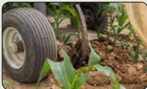
Shovels help lift up the edges of plastic. Adjustable gauge wheels determine the depth of the coulters and shovels.
