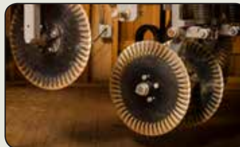
Optional double coulters adapter kit for multiple row beds
