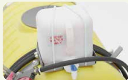
Safety Rinse Tank
